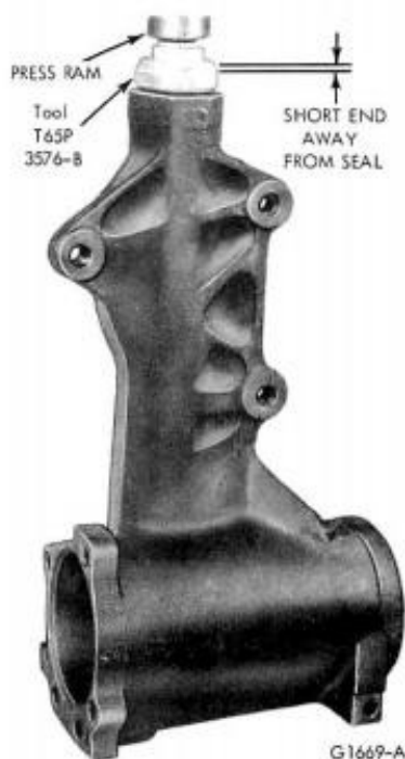
FIG. 21—Installing Sector Shaft Inner Seal
