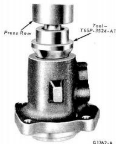
FIG. 18—Installing Oil Seal in Valve Housing
